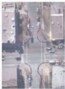
Corner Bulges (width of side street is 33ft)
